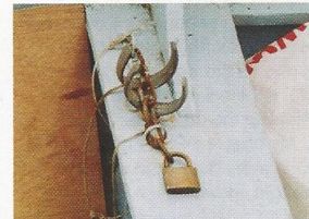
Lock and chain the rowlocks in between two strong U-bolts
