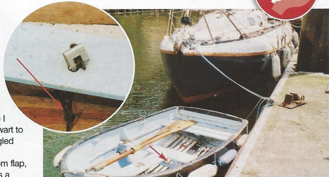
Oars with holes can be chained and padlocked to the thwart (inset) or use a hinged transom to slide them through a bracket under the thwart
