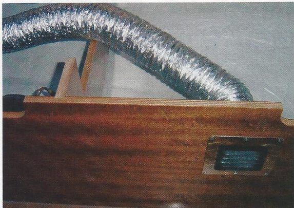
All the bulkheads in my boat had already been cut away in the factory, so the flexible central heating ducting could be threaded through very easily
