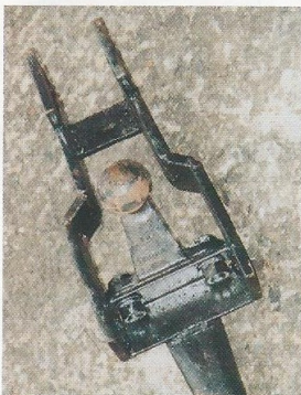
A standard ball-hitch is bolted to the bar and the sturdy side cheeks and strap are welded into position. These allow controlled vertical movement
