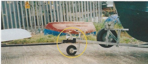
The raised side cheeks keep it straight as the trailer pivots down the slipway
