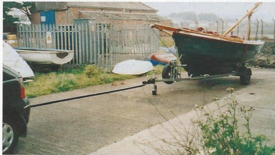
The draw bar extension allows the car to stay on firmer dry land
