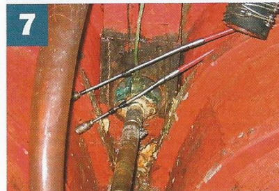
7 Disconnect the prop shaft. You'll have to lie across the engine – this took a long time, made for some well-barked knuckles and a heck of a lot of patience was needed to split the coupling and then remove the machine screws. Although my prop shaft can't fall out, because the propeller is in a cutout in the rudder, I nevertheless have two Jubilee clips clamped on (with screws on opposite sides to keep a balance). The toughest bit was getting the recessed bolts out using a large Allen key
