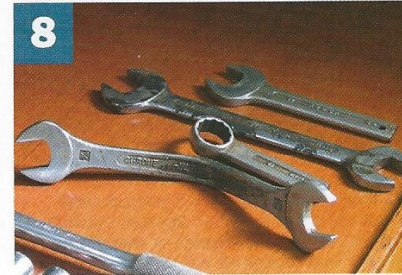
8 The final job was to undo and remove all six engine fixing bolts, or, in this case, 12mm s/s studding, which went right through the longitudinal bearers and the only way of getting at the nuts on the bottom was with some 'doctored' spanners (which thoughtfully came with the boat). Several nuts went into the muck in the bottom of the bilge to be retrieved at clean up
