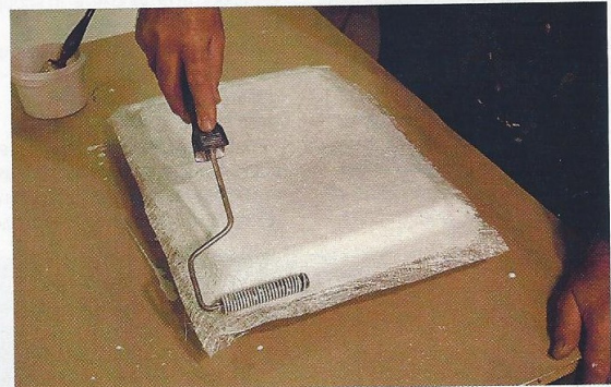
▲ To squeeze out any air bubbles and properly incorporate the chopped strand mat into the resin, you'll need a special consolidation roller. The most effective all-purpose types are made from detachable steel washers
