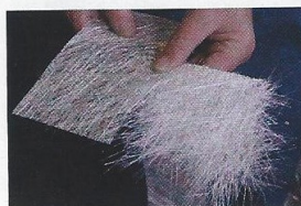
▲ Chopped strand mat (CSM) comes in two forms: emulsion-bound (left), and powder-bound (right)
