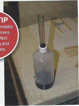
▲ Special dispensers are available for the safe decanting of catalyst, but syringes or eyedroppers are also suitable for the purpose
