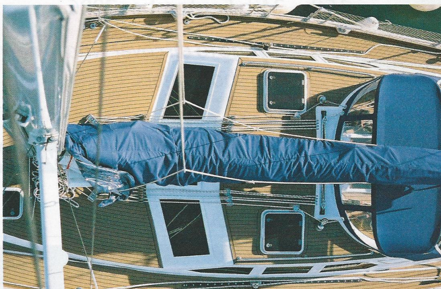
▲ Artificial teak is UV stable, as proved by the 10-year-old Tek-Dek on this yacht in the south of France
