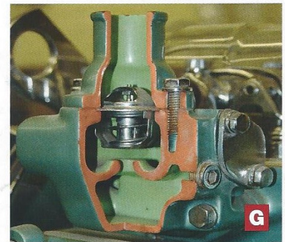
Cutaway engine showing thermostat
