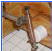
Bronze rod drilled and tapped
